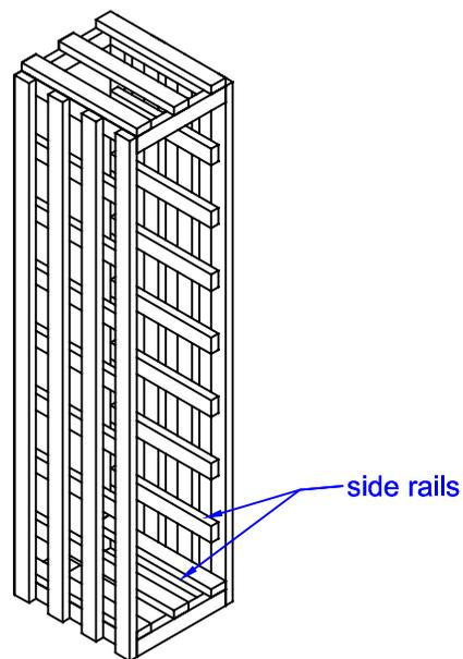
3. Keep adding shelves from the bottom up and nailing them on. Securing the top last.
