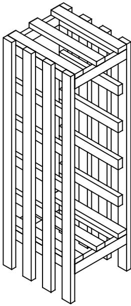
2. Nail only the bottom shelf to the side rail. Leave the top shelf to keep the spacing.
