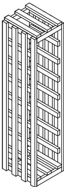
2. Nail only the bottom shelf to the side rail. Leave the top shelf to keep the spacing.
